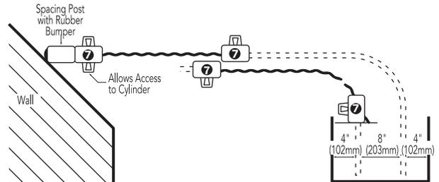
For use when minimal pocket depth is available. A top and bottom lead post with attached spacing post to an angled wall allows access to locking on the acute angle side.
