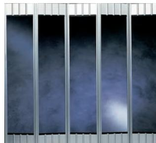
Curtain: 11 1/4" (286 mm) wide-body panels with 1/8" (3 mm) thick fire-retardant polycarbonate that fit into aluminum hinges. Panels are framed by min. 4" (102 mm) high aluminum bottom plates and 5 1/4" (133 mm) high aluminum top plates. Visibility: 100% of 8 7/8" (225 mm) viewable area\*.
