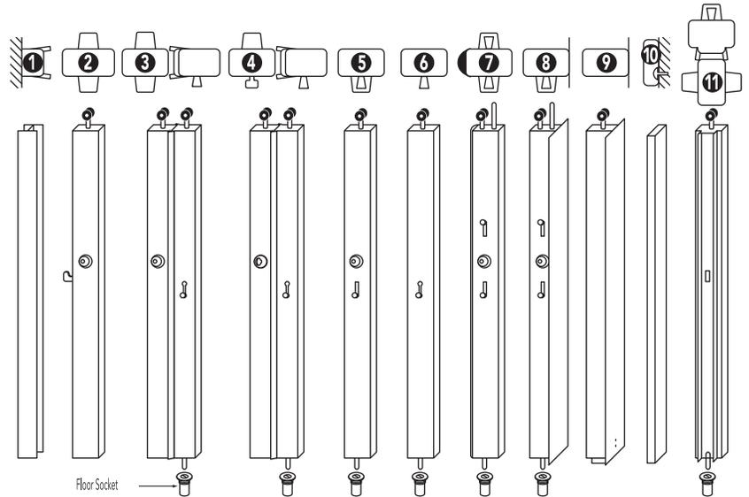
**Single stack into pocket with wall channel or pocket**
