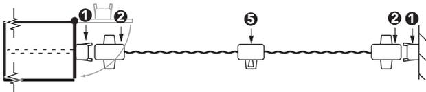
In this configuration, the traveling end post becomes a secured, keyed locking post and avoids drilling for floor socket needed by #7 post.
