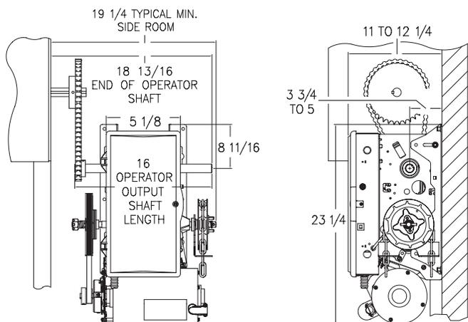
Note: For "A" and "G" dimensions, refer to Headroom and Guide Clearance. Dimension charts applicable to grille type selected.
