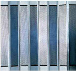
Curtain: 7" (178 mm) standard-width, 18-gauge painted perforated steel panels with 3/16" (5 mm) dia. holes on staggered centers that slide into aluminum hinges. Panels are framed by min. 4" (102 mm) high aluminum bottom plates and 5 1/4" (133 mm) high aluminum top plates. Visibility: 51% of 4 3/4" (121 mm) viewable area.
