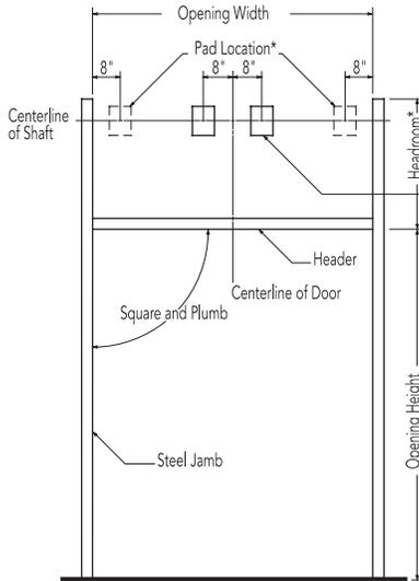
\* Pad Location for additional shaft support brackets for doors over 18'3" wide
